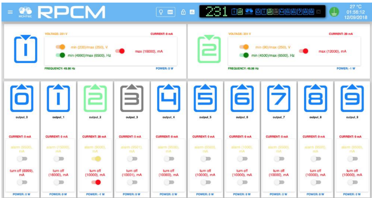
Figure 4.2.18. The Dashboard control panel in the Show Limits mode RPCM 1502 and RPCM 1532 with the switches on the inputs and the 2nd output turned on.
