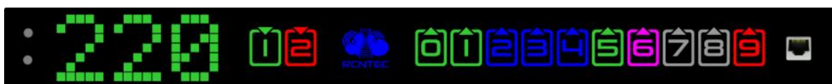
Figure 3.1.1. The draw of the display panel with control elements and Ethernet ports for RPCM with ATS: RPCM 1502 or RPCM 1532.
