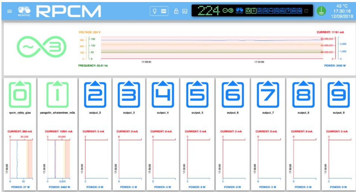
Figure 4.2.23. The Dashboard of RPCM 3x250 "View Mode" with the Show Limit activated.
