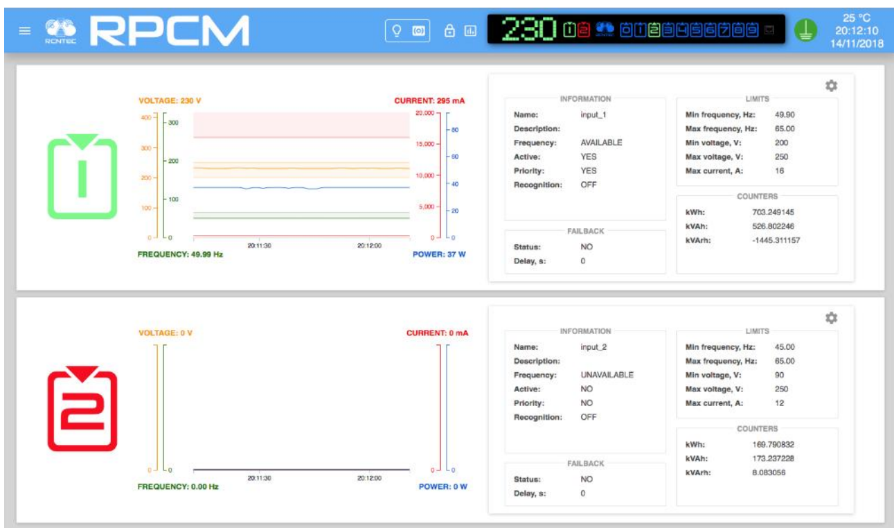
Figure 4.4.12. Showing Current Limits for the first input is on (RPCM 1502 and RPCM 1532).
