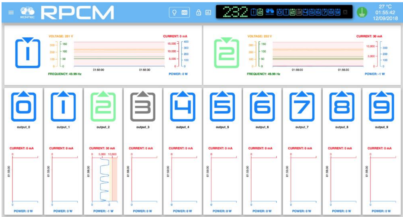
Figure 4.2.21. The Dashboard control panel in the "View Mode" with the Show Limits mode enabled.
