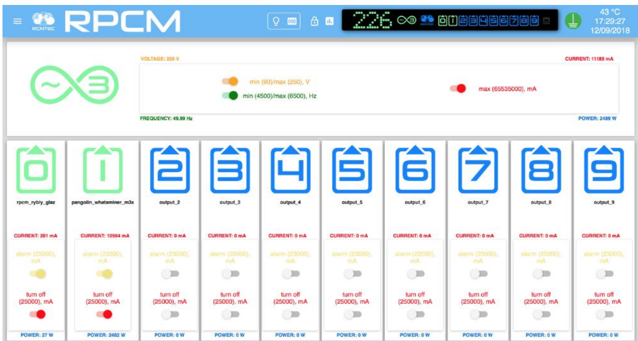
Figure 4.2.22. The Dashboard in Show Limit configuration mode for RPCM 3x250 with the limit switches of the input and 0 and 1 outlets turned on.
