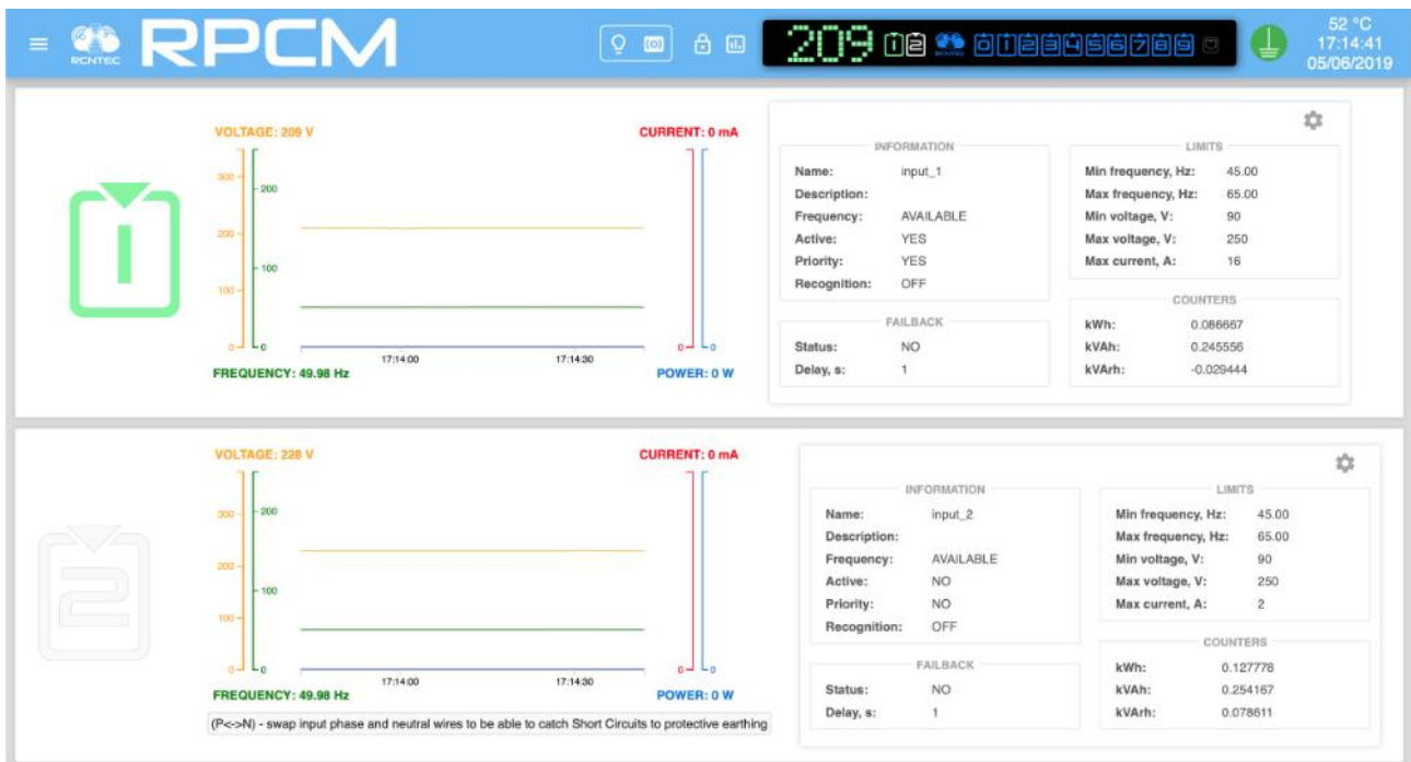
Figure 4.4.14. When notifying about the incorrect (inverse) connection is on, the inputs number is blinking.
