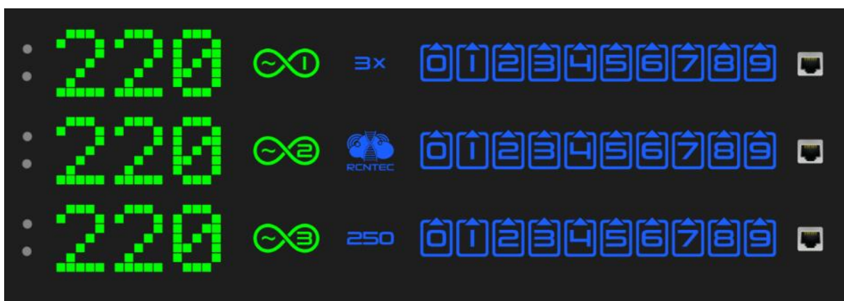
Figure 3.1.2. The draw of the display panel with control elements and Ethernet ports for RPCM 3x250.
