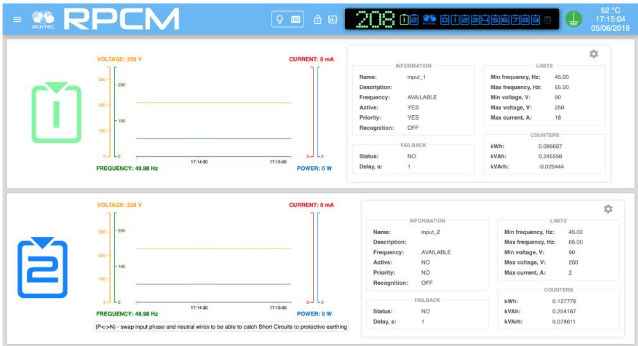
Figure 4.4.13. Notification of incorrect (inverse) connection at input "2".
