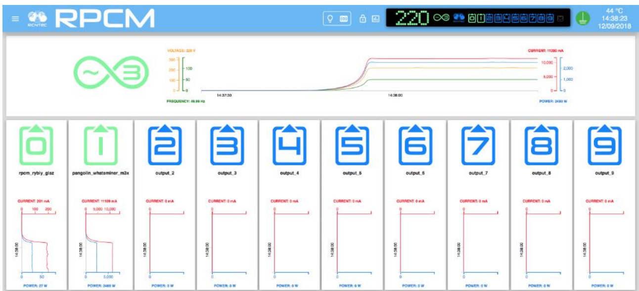
Figure 4.2.15. The Dashboard control panel of the RPCM 3x250 module #3 in the View Mode.
